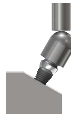
30° Fatigue testing ISO 14801
